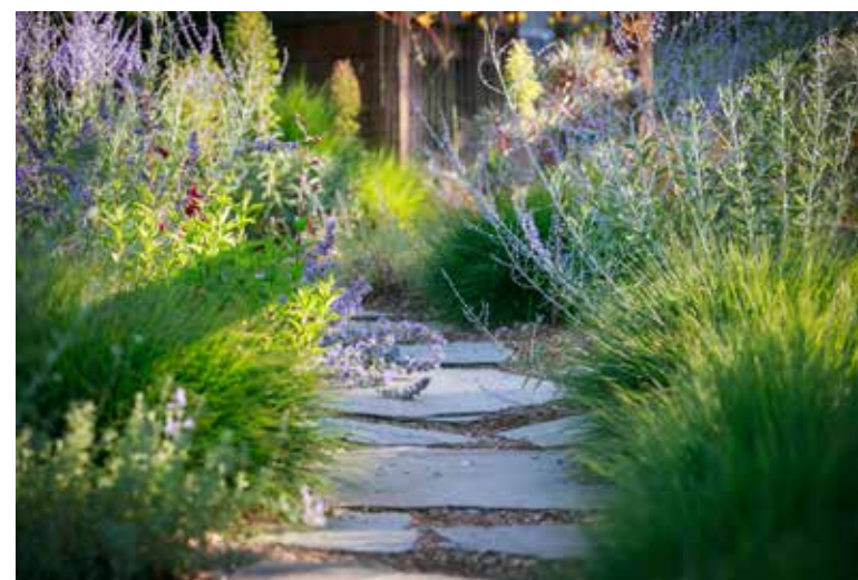
In addition to the flagstone walkway, crushed rock and permeable hardscape surfaces were used to reduce the amount of surface water runoff as well as the number of impermeable surfaces. Drought-tolerant and California native plants were used to reduce water consumption.
